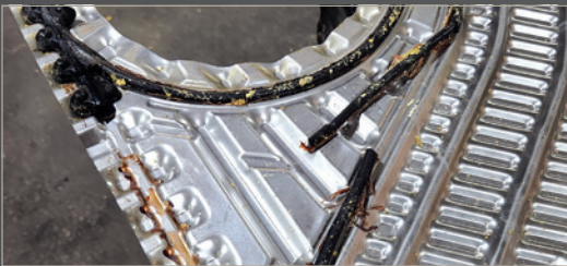
Damaged bridge gaskets
